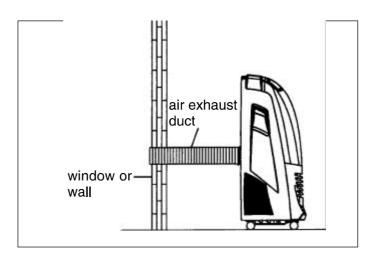
If this unit is ONLY used as a dehumidifier, always remember to remove the air exhaust duct from the main unit. When used as a air conditioner, mount the air exhaust duct to the air outlet (terminal) of the main unit.
