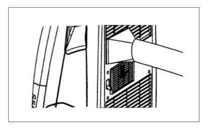
Correct mounting shown below (If mounting in the wall, the height of the hole should be 40cm ~ 130cm)
