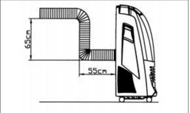
The wrong mounting diagram (Air exhaust bend too large, easily cause malfunction).
